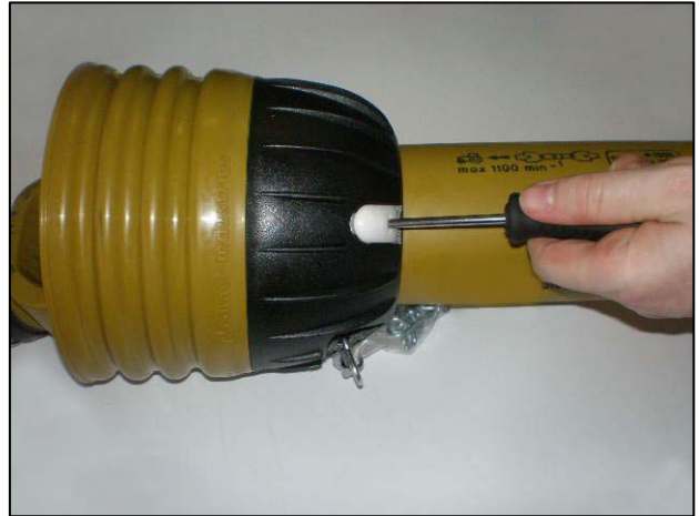
Insert screwdrivers into the clasps
