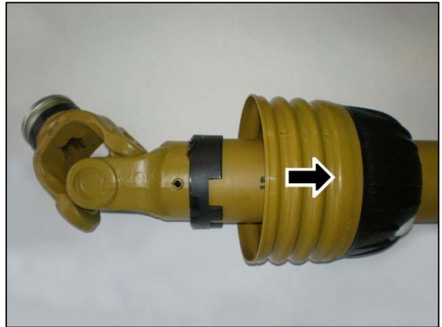
Slide shield back to reveal universal joint
