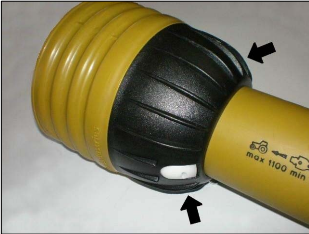
Shaft shield fixing clasps
