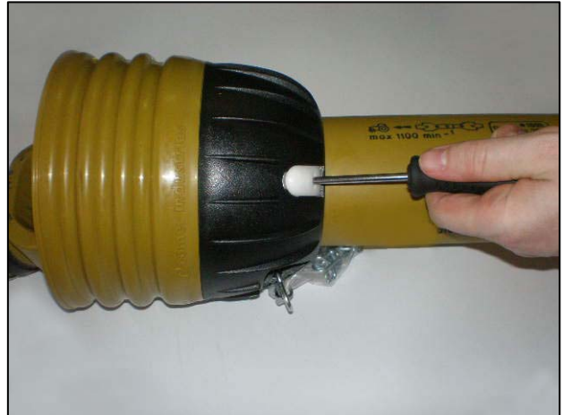
Insert screwdrivers into the clasps
