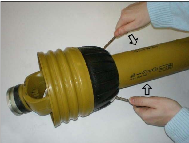
Prise clasps open to release the shield
