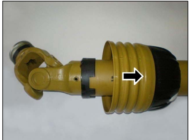
Slide shield back to reveal universal joint
