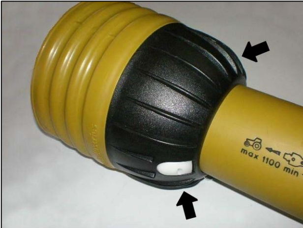
Shaft shield fixing clasps
