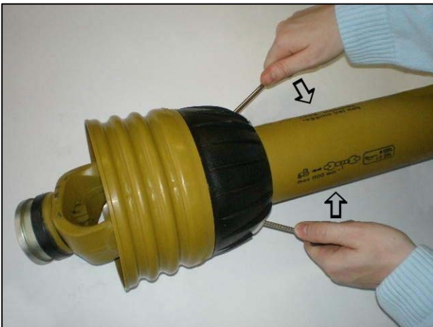
Prise clasps open to release the shield
