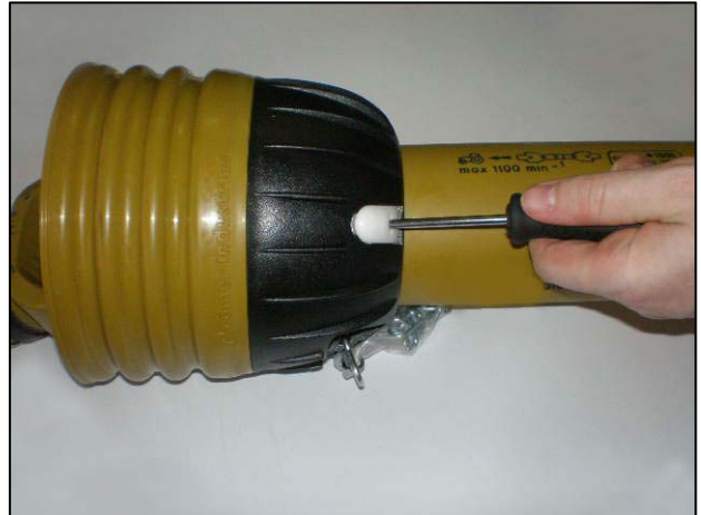
Insert screwdrivers into the clasps
