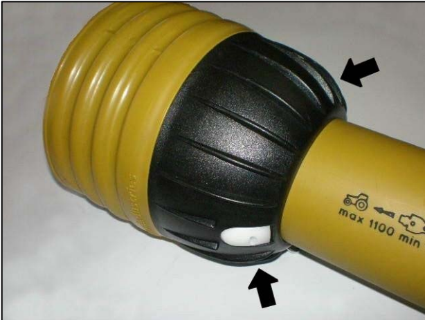
Shaft shield fixing clasps
