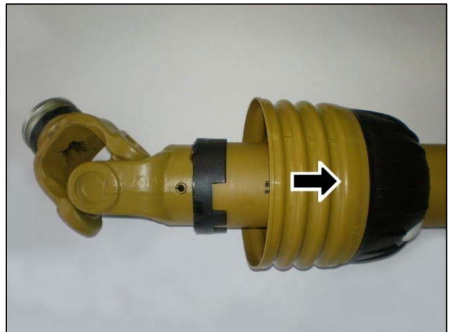
Slide shield back to reveal universal joint
