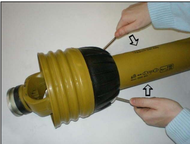
Prise clasps open to release the shield
