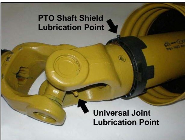
Location of lubrication points
