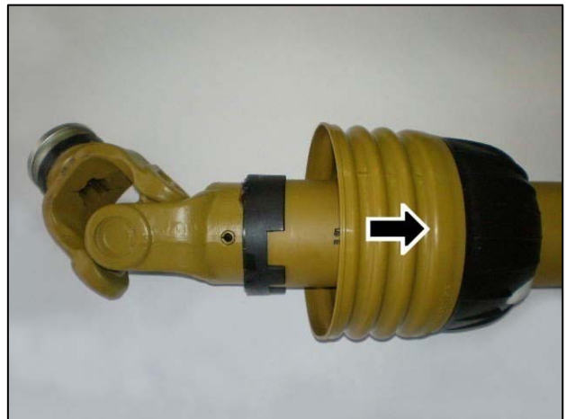
Slide shield back to reveal universal joint
