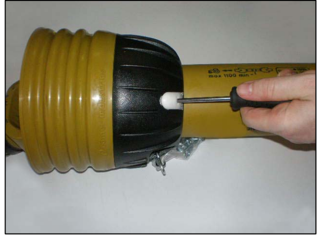
Insert screwdrivers into the clasps
