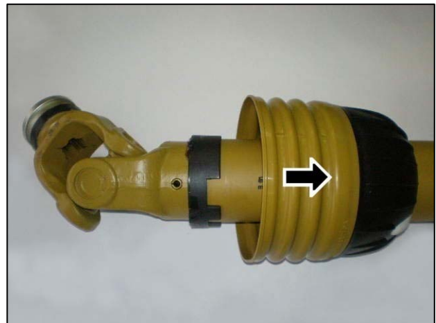
Slide shield back to reveal universal joint
