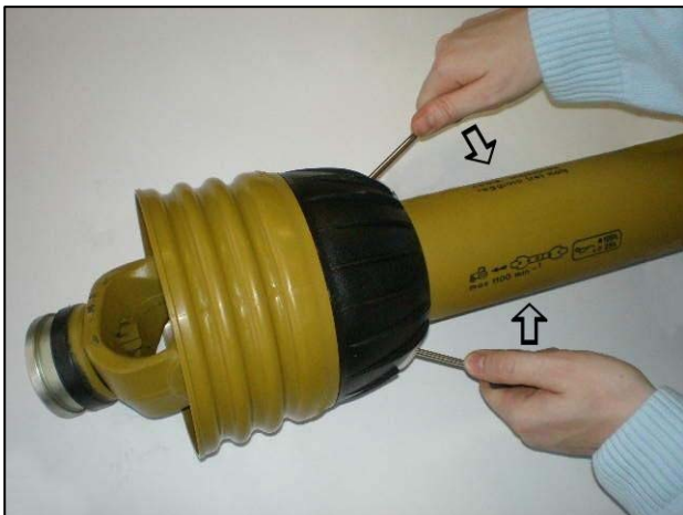
Prise clasps open to release the shield
