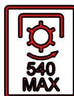
Frequency and direction of rotation of PTO input shaft
