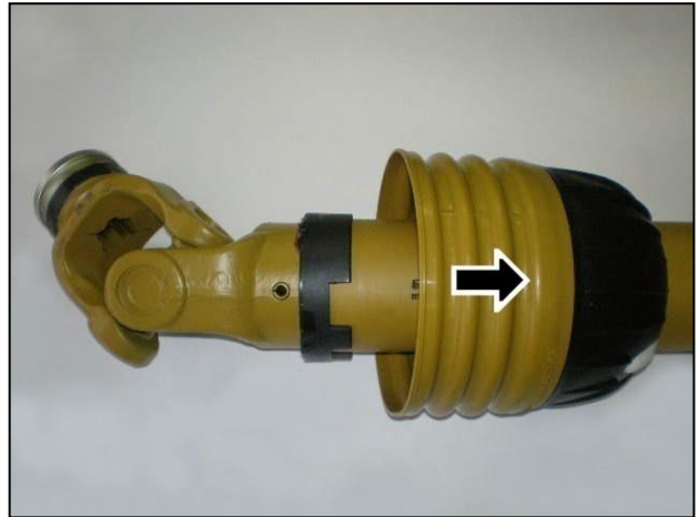
Slide shield back to reveal universal joint
