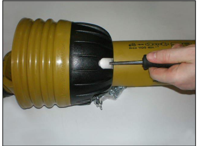
Insert screwdrivers into the clasps
