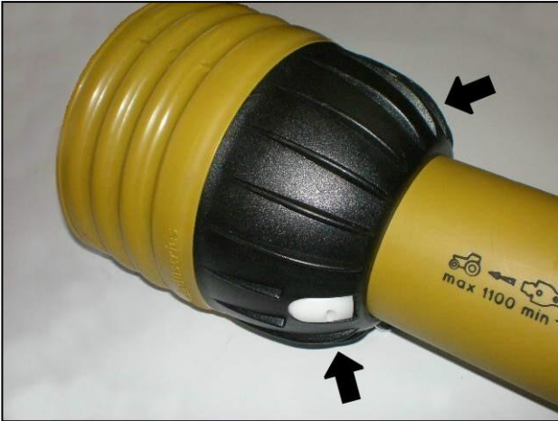
Shaft shield fixing clasps
