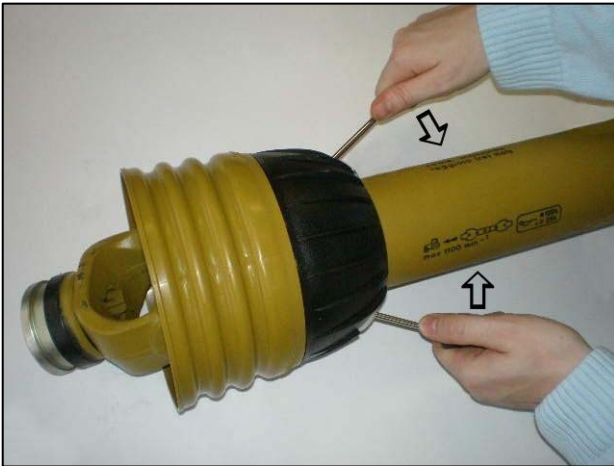
Prise clasps open to release the shield
