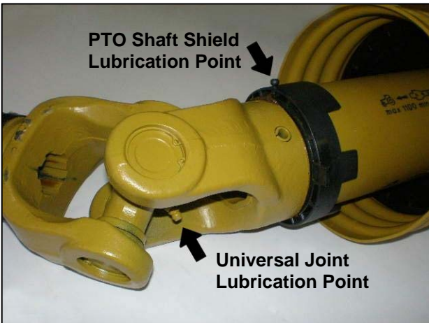
Location of lubrication points
