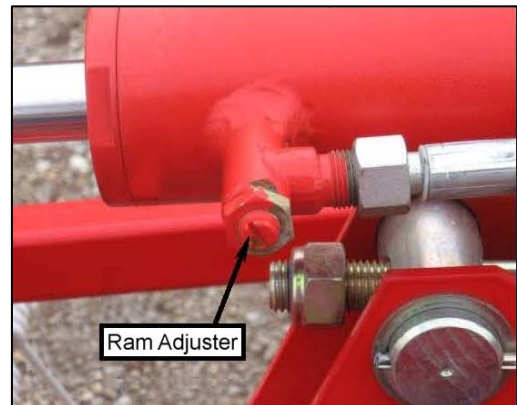
Moving into transport position – raise right hand wing first. Ram speed can be altered with adjuster.
