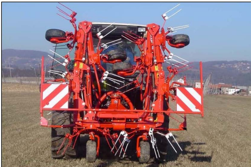
Transport Position – check wings are fully latched in the transport lock
