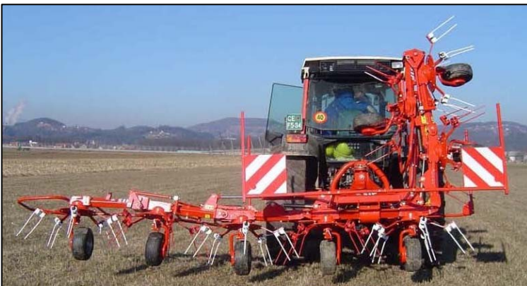
Moving into transport position – raise right hand wing first. Ram speed can be altered with adjuster.
