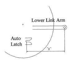
First set tractor link arm so that it is horizontal, then measure the horizontal distance between the centre of the lower link eye and the centre of the Auto latch, distance 'X'.
