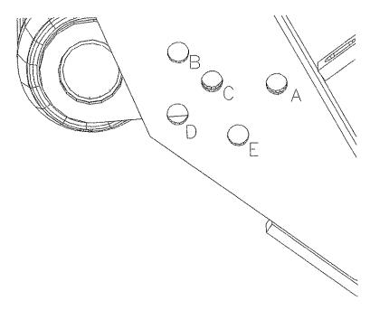
Bolt position A is the main pivot position, about which the roller bracket will normally pivot. From the pivot position A, the second bolt can be put in any of the positions, B, C, D or E. This sequence B to E is that from shortest to longest cut length.
