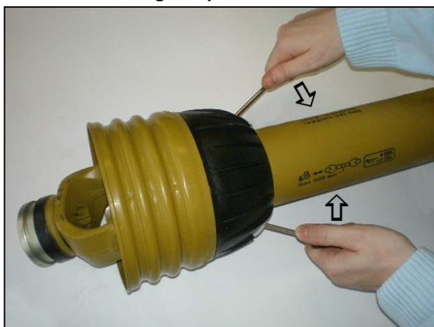
Prise clasps open to release the shield
