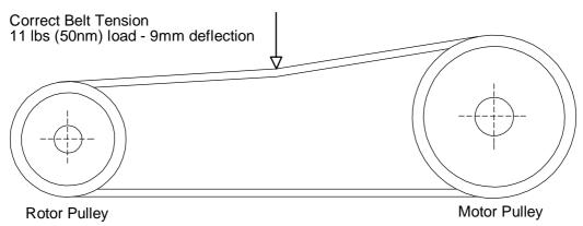
• When belts have been tensioned correctly and all covers replaced, the machine is ready for start up.
