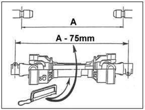
Measure the PTO shaft and cut to the dimension shown – the finished length of the PTO shaft should be 75mm (3") less than the measured distance 'A' -between tractor shaft and gearbox stub shaft – to enable fitting. NOTE:
