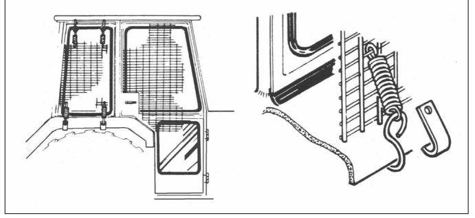
Use a tractor with 'safety glass' windows if possible and fit **Operator guard** (*Part No.7313324*) using the hooks provided.
