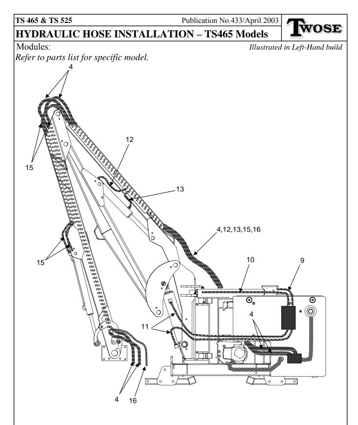
The illustration above serves only as a general guide to hose positions and locations, it is therefore advisable when replacing hoses to run the replacement alongside the old one prior to removal to ensure the correct route and location.
