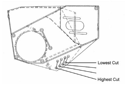
To alter the roller position, each end bracket of the roller and the relative securing bolts will need to be positioned at either of the four position height options offered. Ensure that same opposing location holes on the flail head are chosen.
