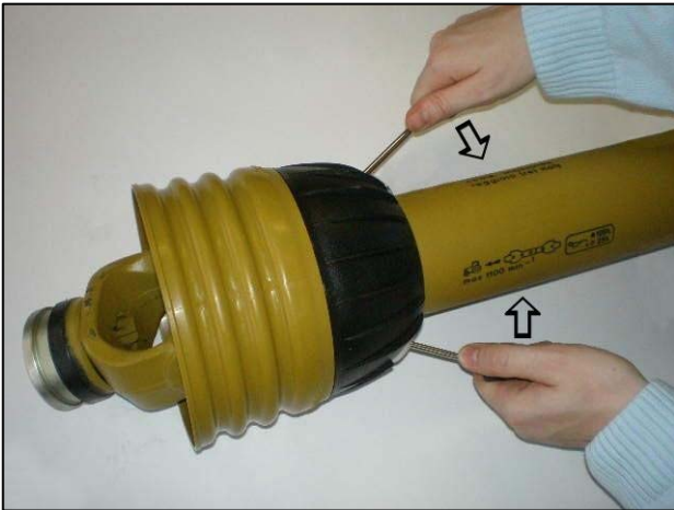
Prise clasps open to release the shield
