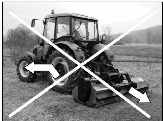
Raise the machine before turning or reversing
