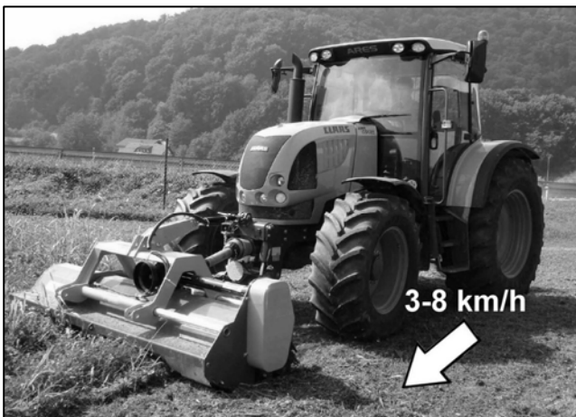
Optimal forward working speed 3-8 km/h
