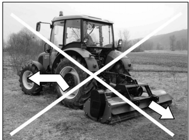
Raise the machine before turning or reversing
