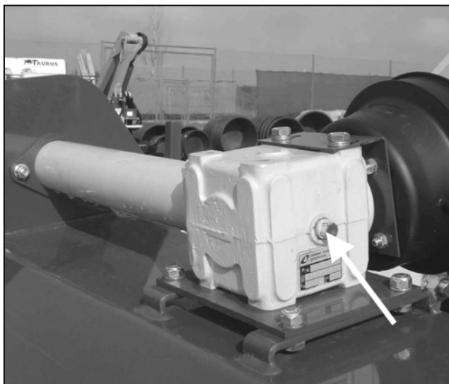
Location of gearbox lubricant access plug
