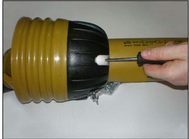
Insert screwdrivers into the clasps
