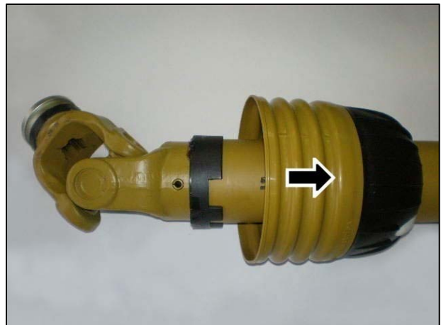
Slide shield back to reveal universal joint
