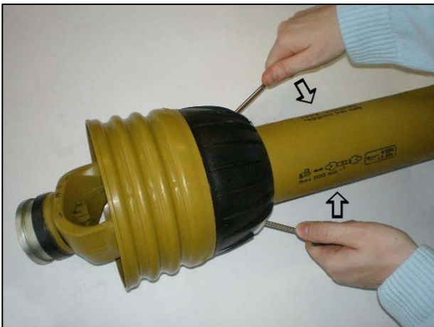
Prise clasps open to release the shield
