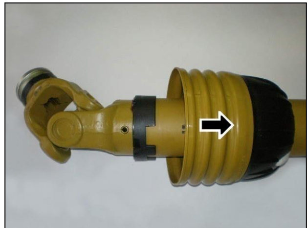
Slide shield back to reveal universal joint
