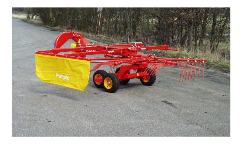
Rotary Side Delivery Rake
