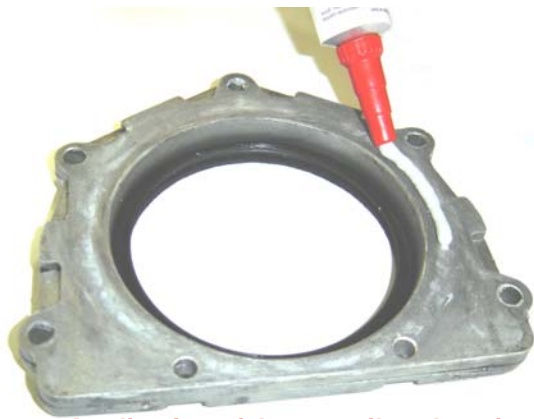
Application of the rear oil seal retainer junction
