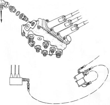
The plug from the end of the pressure gallery on the armhead control valve is removed and replaced with a pressure carry over adaptor, a union and a swivel elbow. The pressure supply to the debris blower is taken from this swivel elbow to the flow control valve block on the blower motor opposite the hexagon head of the valve.
