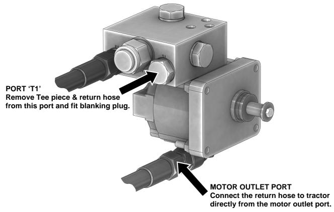
The Tee piece, the long return hose to the tractor and the short return hose from the motor outlet port should be removed from port 'T1'.
