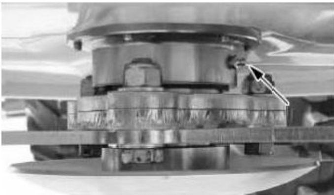
Bearing lubrication point
