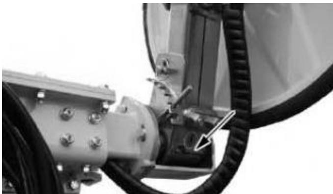
Rotor support arm lubrication point
