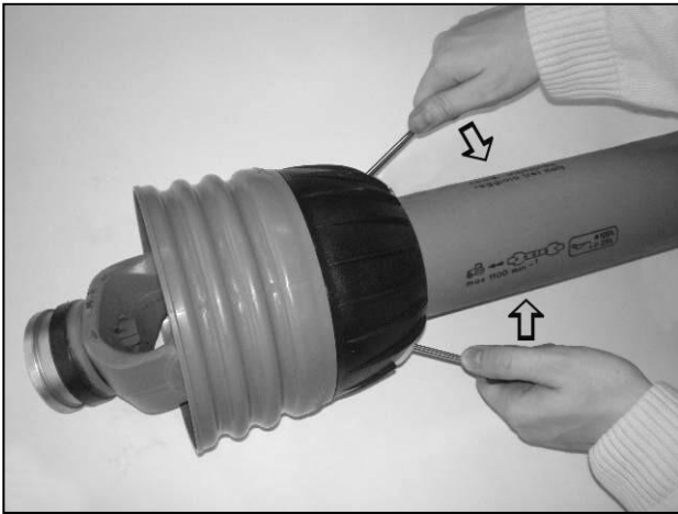
Prise clasps open to release the shield
