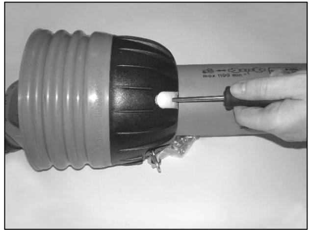
Insert screwdrivers into the clasps
