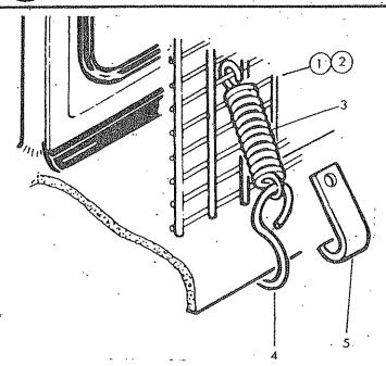
Ref. Part No. Qty. Description 73 13 324 CAB GUARD KIT Guard panel - large Guard panel - small 73 13 049 73 13 050 1 3 60 01 064 Spring 12 Hook 60 01 065 73 13 051 6 .Hook CONTROL MOUNTING ASSEMBLY 71 09 319 71 09 146 Pillar 93 11 086 Setscrew 01 11 006 Nut 01 00 206 Spring washer
