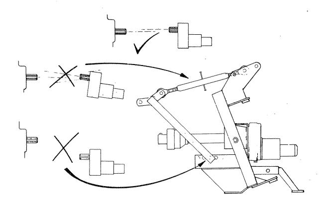
Tighten up the check chains or adjustable stabilisers to hold the machine rigid with out side-sway.
