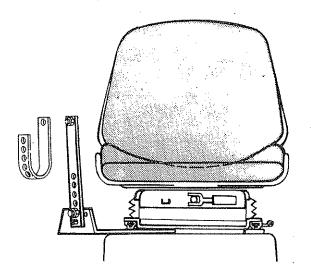
Illustration shows control unit arrangement for fully independent model with extra control handle for rotor ON - OFF. This handle can be mounted either end of the main control block to suit individual operator requirements
