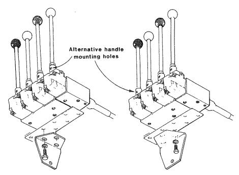
The control unit itself is bolted to an angled mounting bracket in either a transverse or longitudinal position thus giving a variety of mounting positions, which in conjunction with the flexibility of the mounting pillar will enable a satisfactory working position to be achieved.
