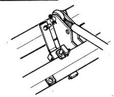
The arm can then be returned to the work position by either reversing the tractor or by operating the 'lift' control to raise the head which allows the breakaway mechanism to position the flail head for work.
