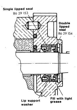
The seal kit, Part No. 86 99 166 is a universal Cassapa motor sealkit. It may contain more seals than are necessary; care must be taken in selecting the correct seal to use.
