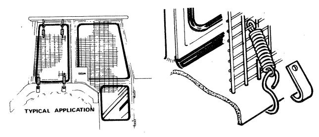
Polycarbonate transparent sheeting is an impact resistant material which can be readily sawn and shaped to requirements. Unfortunately it is susceptible to surface damage and scratching, therefore it is advisable to place the material on the inside of the window for protection. No attempt should be made to wipe the sheeting with dirt engrained cloth.
