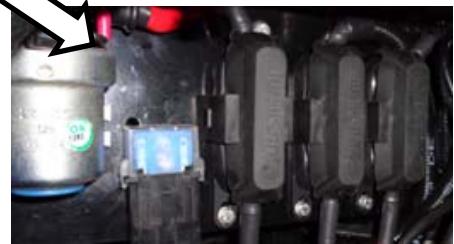
Auxiliary fuse / relays
