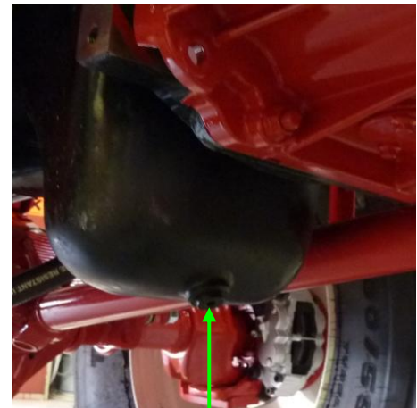
Sump oil drain plug
