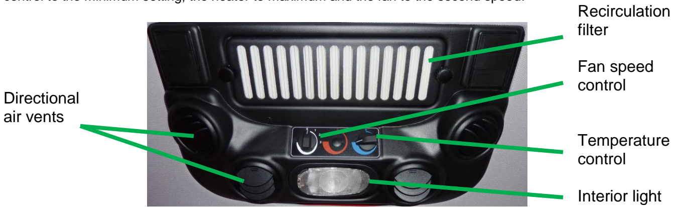
Air conditioning console
