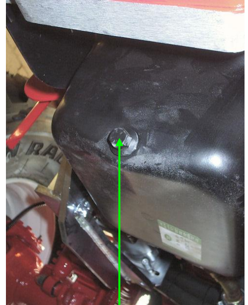
Sump oil drain plug
