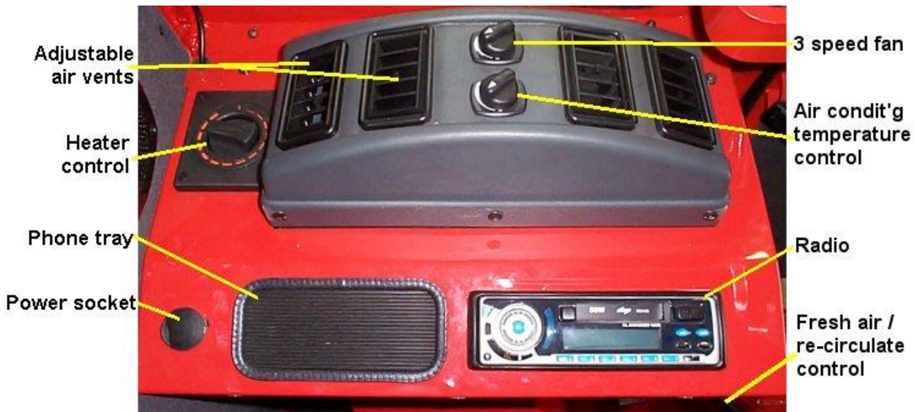
Air conditioning console
