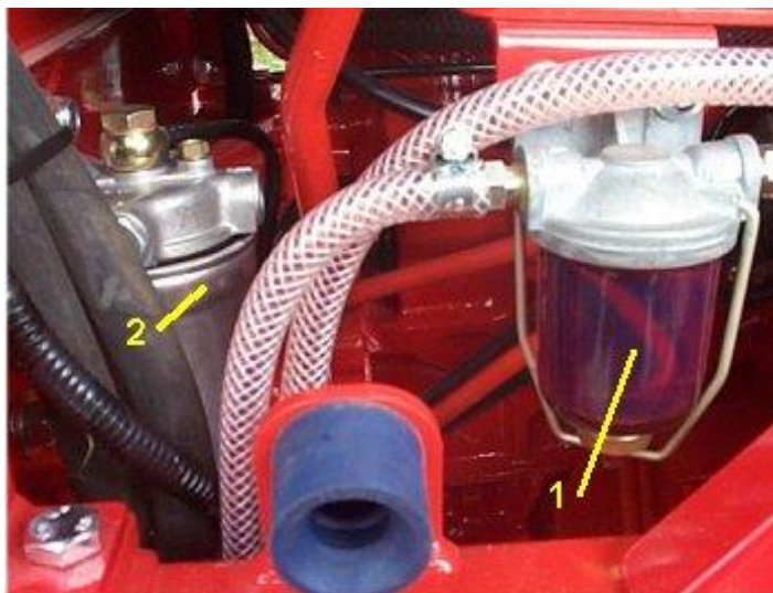
1. Water / sediment trap 2. Fuel filter
