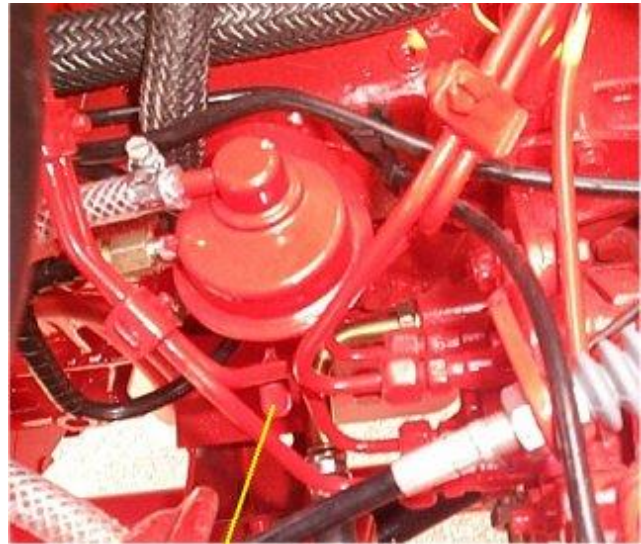
Fuel lift pump lever
