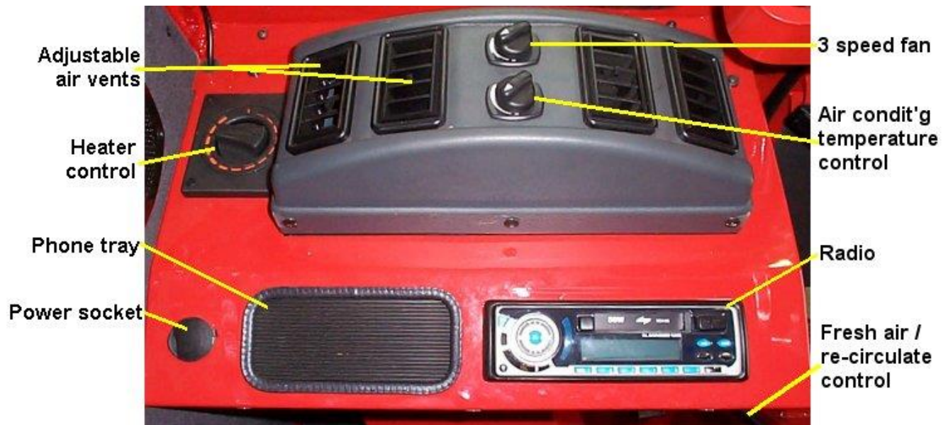
Air conditioning console
