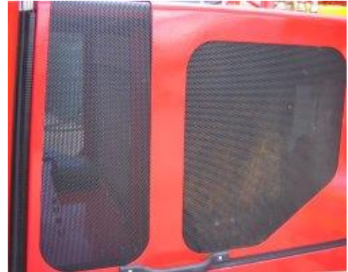
Air intake/outlet grills
