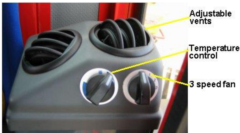
Air conditioning console
