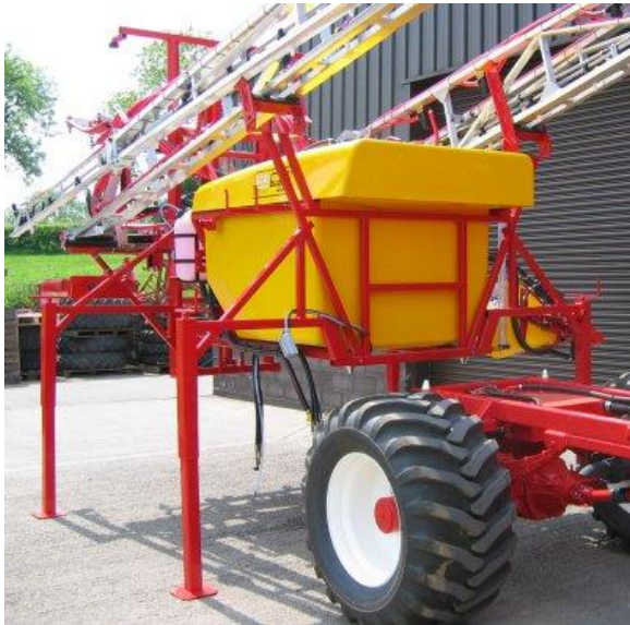
The cone guidance system automatically aligns the demount frame when re-fitting.
