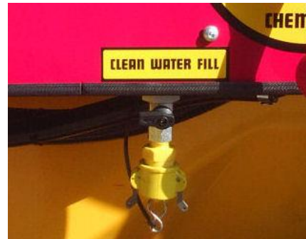
Wash tank connector
