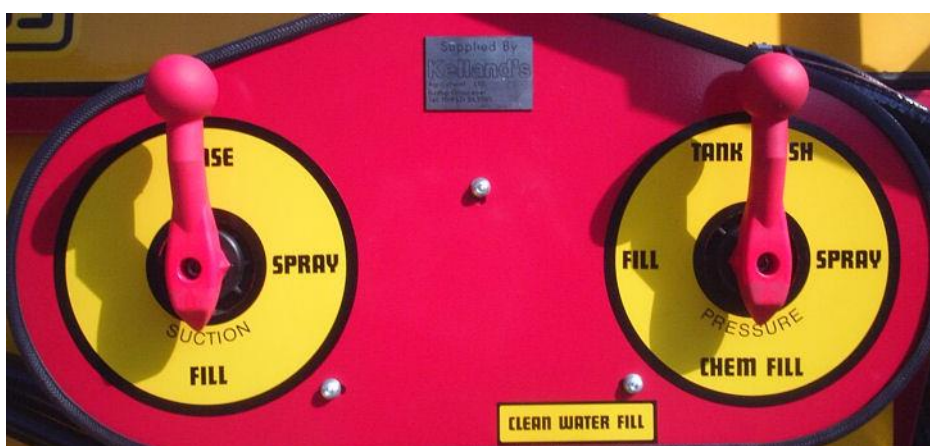
Normal Valve positions whilst using inductor
