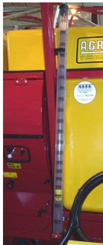
Tank sight gauge
