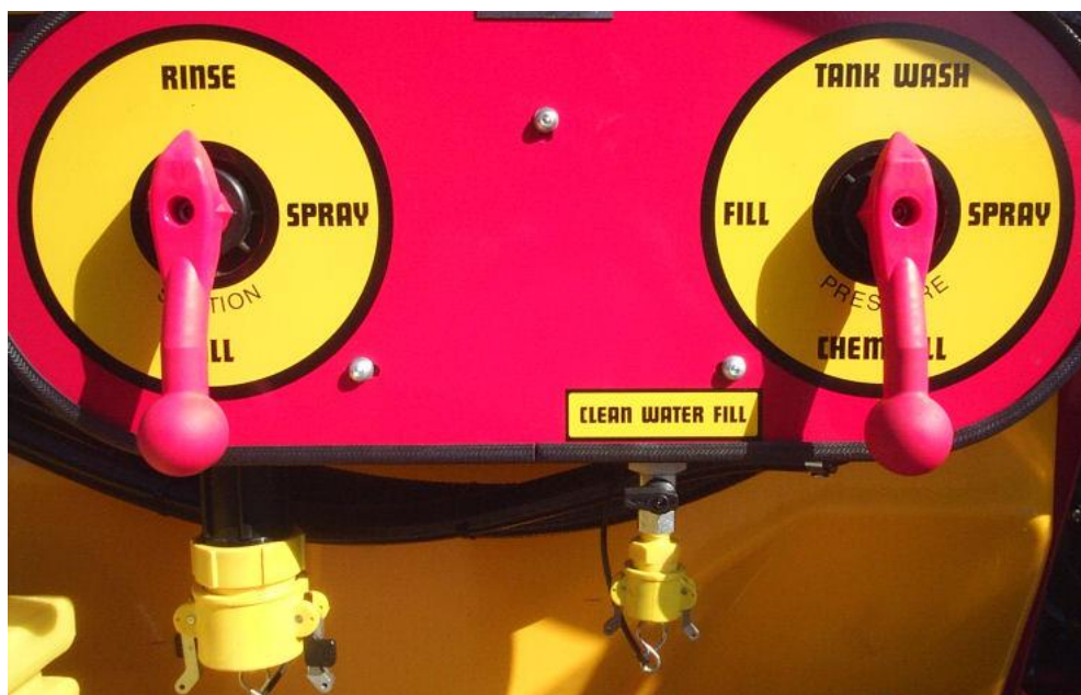
Valve positions for tank washing
