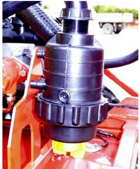
Main suction filter assembly
