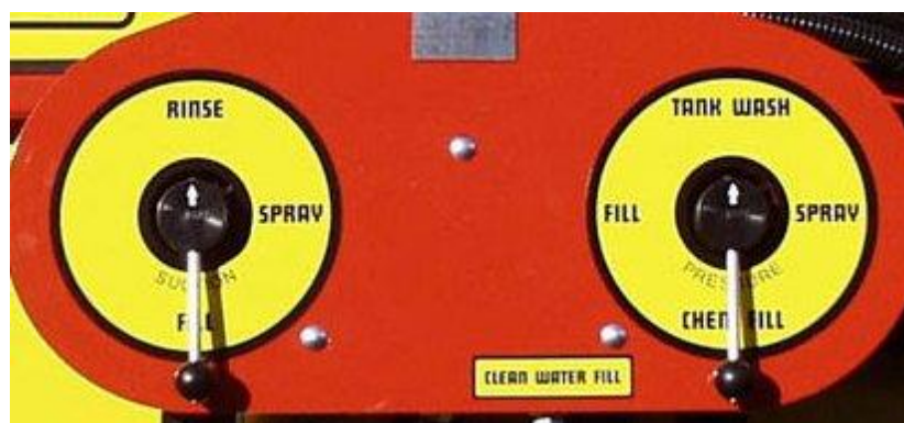
Valve positions for tank washing
