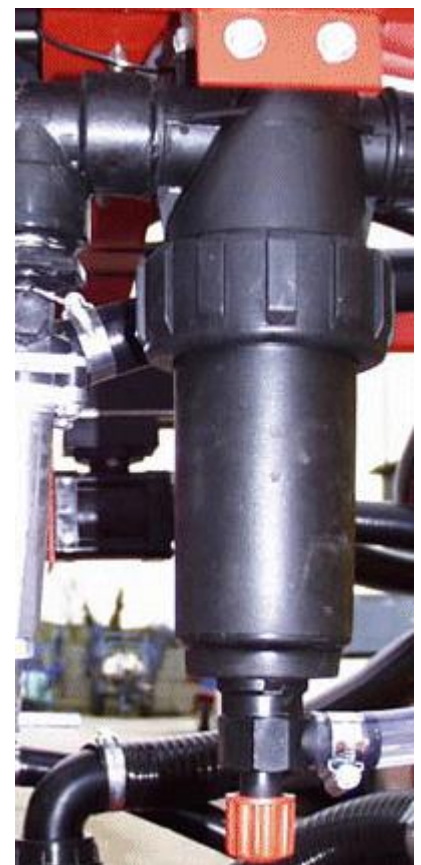
Main pressure filter assy
