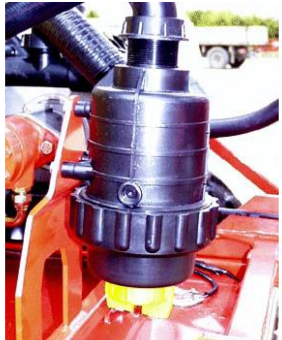
Main suction filter assembly
