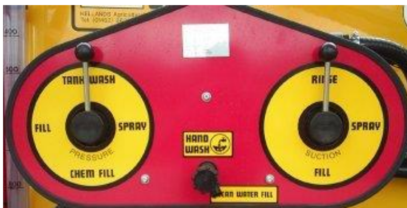
Normal Valve positions whilst using inductor
