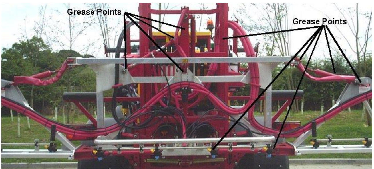
Boom lubrication points
