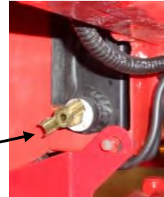
Radiator drain tap viewed from RH side of chassis
