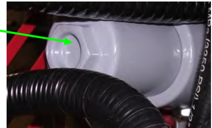
Transmission filter mounted on rear engine bulkhead
