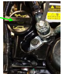
Lubricating Oil Filler Cap Towards the front right-hand side of rocker cover.
