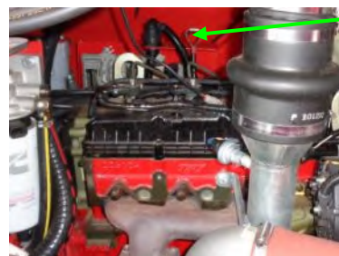
Lubricating Oil Filler Cap Towards the front right-hand side of rocker cover.
