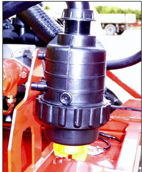
Main Suction Filter Assembly
