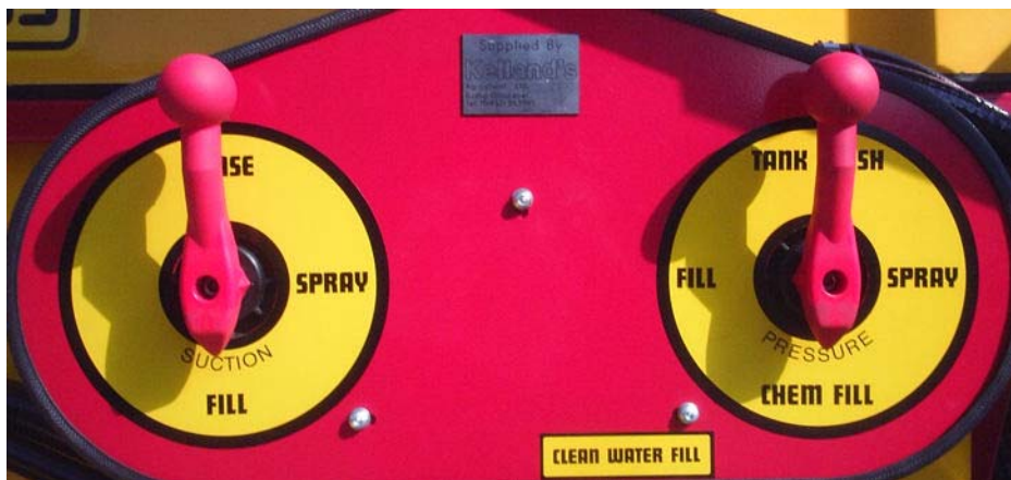
Normal valve positions whilst using inductor
