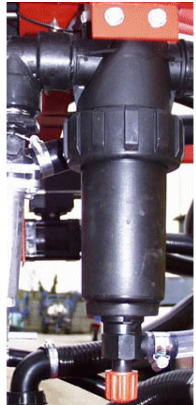
Main Pressure Filter Assembly
