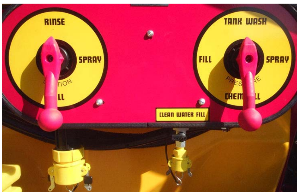
Valve Positions for Tank Washing
