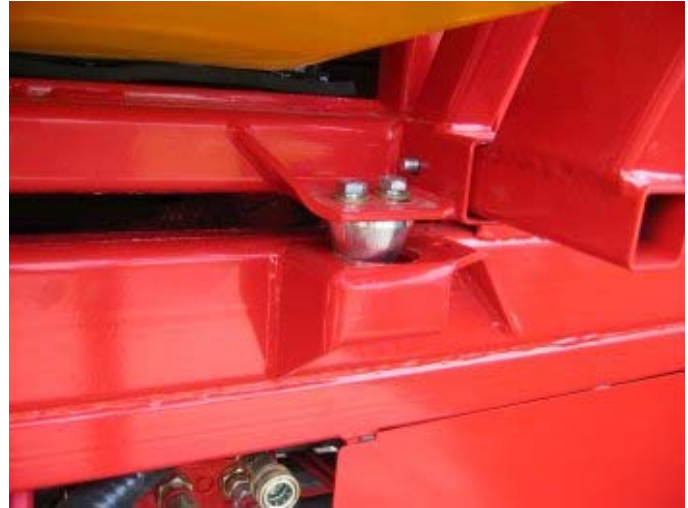
The cone guidance system automatically aligns the demount frame when re-fitting.
