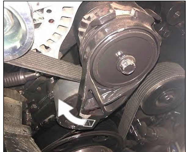
Lever tensioner clockwise to slacken belt
