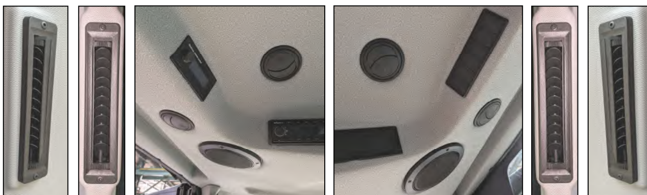
Multi-directional Air Vents are located in roof space and within the cab pillars
