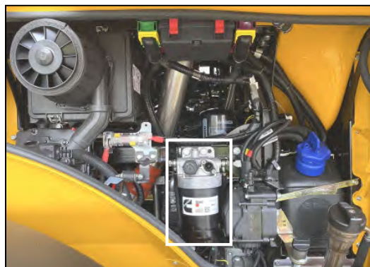
Primary Fuel Filter location
