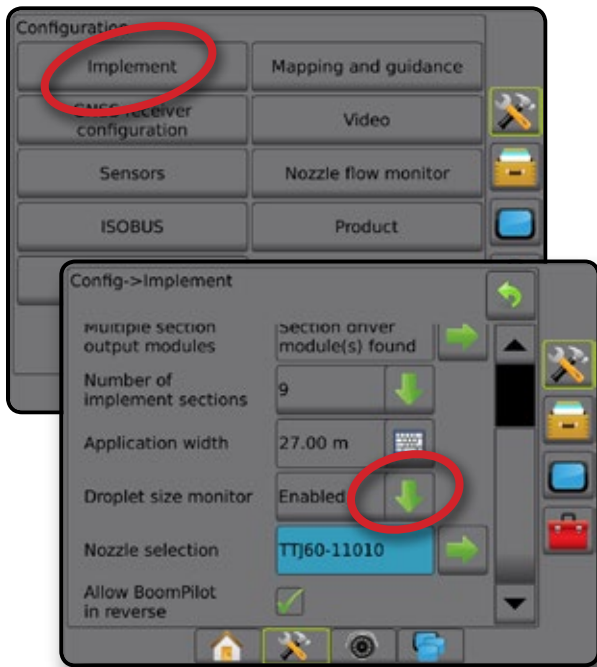
Figure 4-9: Droplet size monitor
