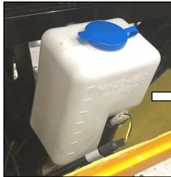
Screen Wash Reservoir
