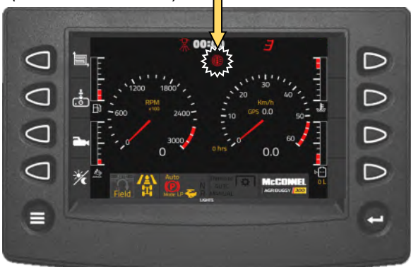
Fast flashing RED Filter Icon: No CAT4 Filter fitted. (1 second flash rate)
