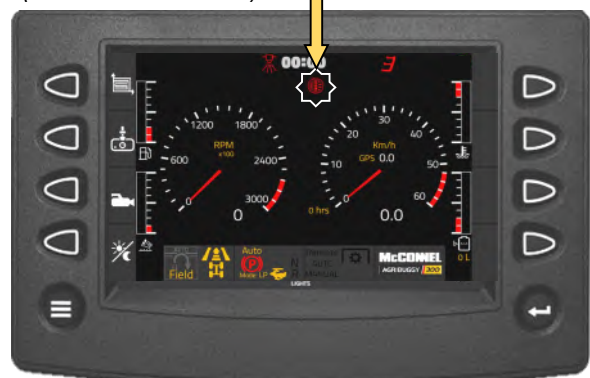
Slow flashing RED Filter Icon: Filter requires replacing (4 second flash rate)
