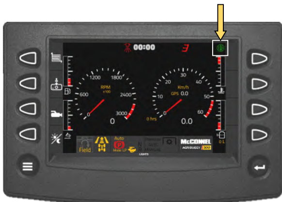
Fast flashing RED Filter Icon: No CAT4 Filter fitted. (1 second flash rate)
