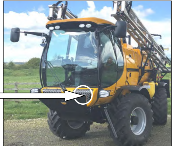
Screen Wash Reservoir Location
