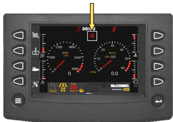
Slow flashing RED Filter Icon: Filter requires replacing (4 second flash rate)
