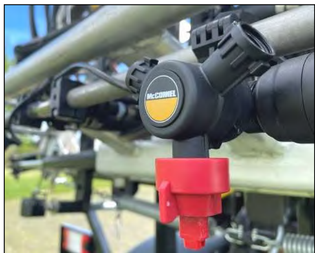
Nozzle Body with Air Activated Check Valve
