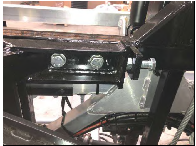
Top Slide Frame Adjusting Bracket
