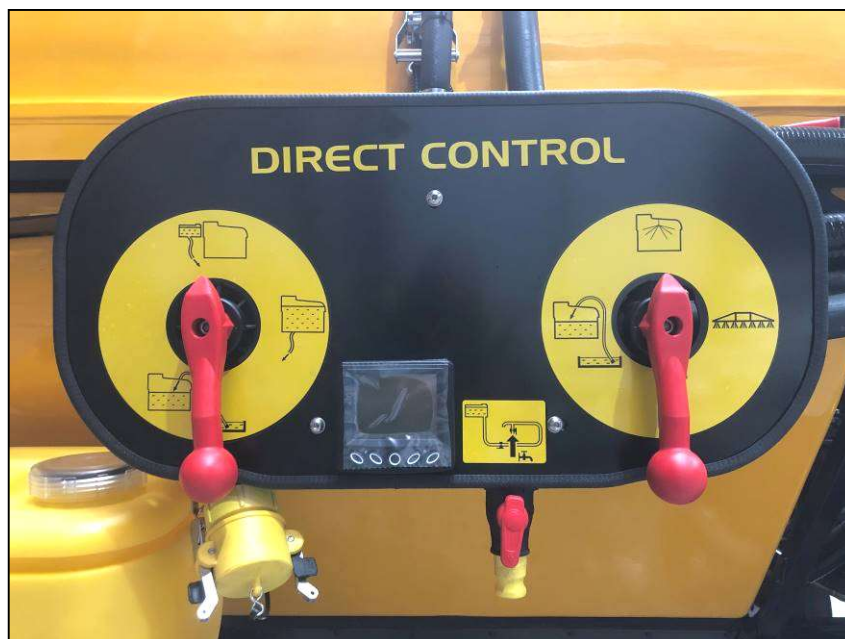
Valve Positions for Tank Washing
