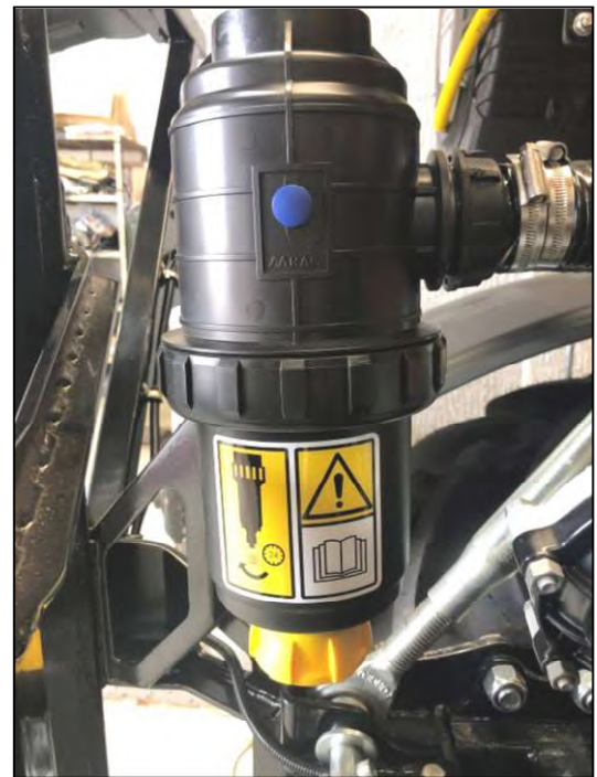
Main Suction Filter Assembly
