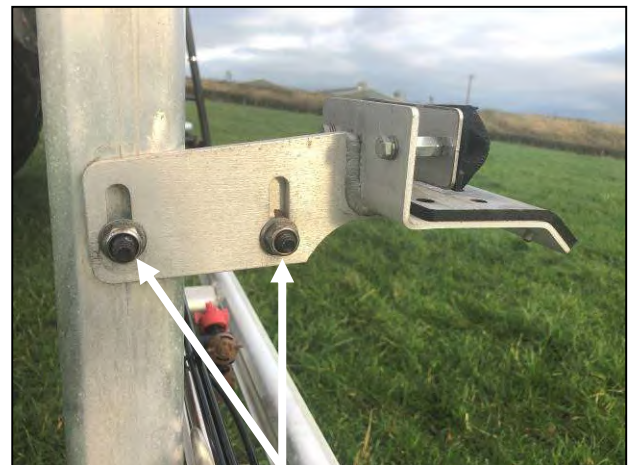
Outer Boom Rest Adjusting Bolts
