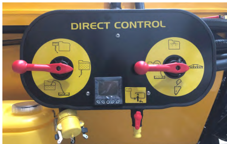
Main Valve positions for spraying/circulating
