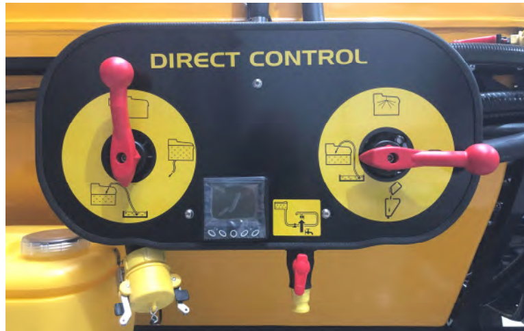
Main Valve positions for water self-filling
