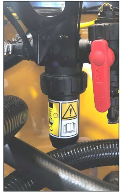
Main Pressure Filter Assembly
