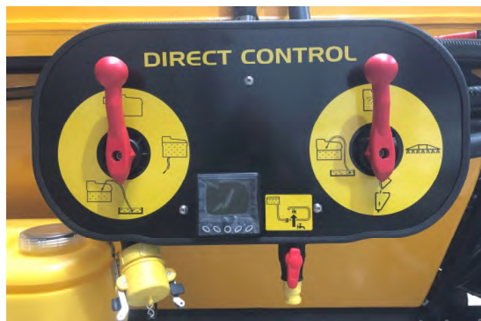
Normal valve positions whilst using inductor
