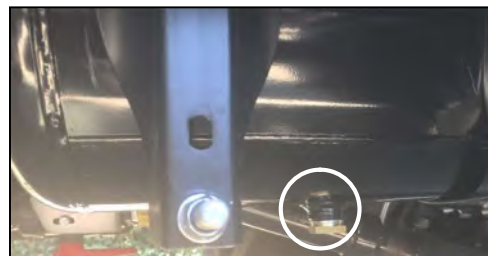
Air Tank Auto Drain Valve
