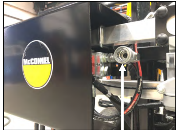
Passive Charge Hose Coupling
