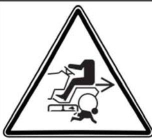
Back Over Hazard
