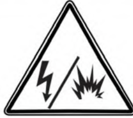
Strike and explosion Hazard Blades Contacting Utility or Gas Lines
