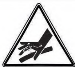
High pressure oil penetrating skin
