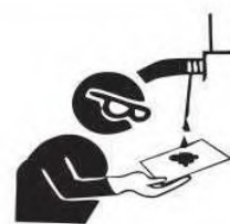
Using cardboard to check for oil leaks
