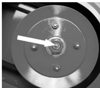
Rotor Bearing Grease Point
