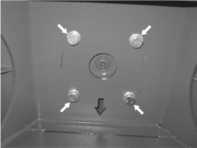
Centre Gearbox Mounting Bolts Location
