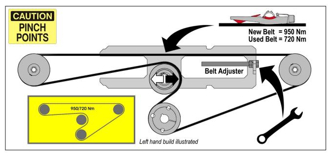
Belt tension is set using the belt adjuster screw on the tensioner assembly. Tension should be checked and measured at the midway point between the pulleys on the longest belt run and adjusted accordingly to achieve correct tension; the correct setting is 950 Nm for a new belt and 720 Nm for a used belt.
