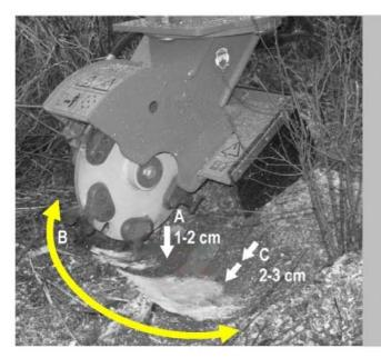
Start the cutter wheel above the stump.
