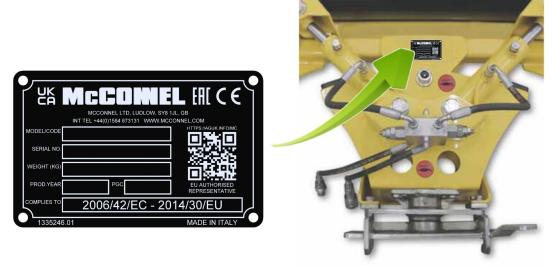
Always quote the machine type and serial number as stated on the identification plate when ordering replacement parts or requesting assistance.
