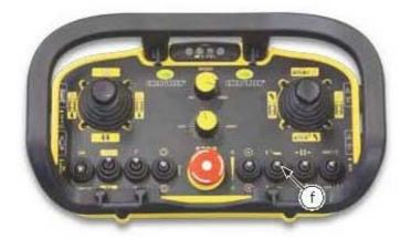
■ Angling of the blade to the left or to the right is controlled by the use of switch 'f' indicated.
