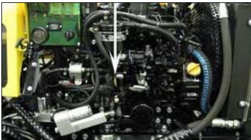
Location of engine oil dipstick
