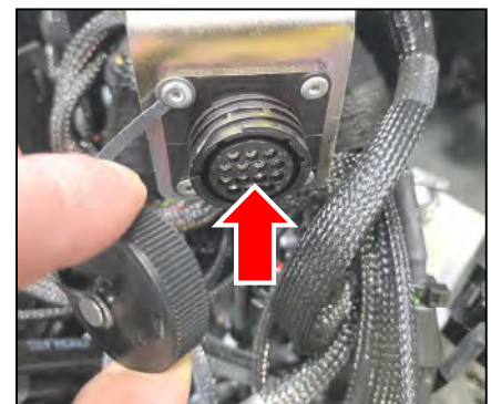
Location and identification of the emergency control unit connection point
