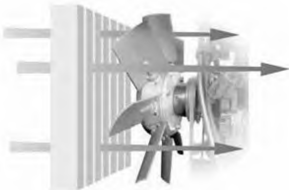
Airflow through radiator for cooling
